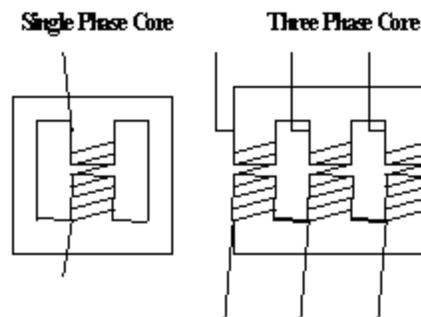
Fig. 8 - Typical Iron Core Designs
