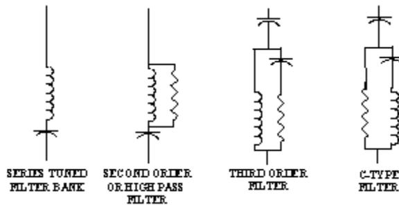
Fig. 3 - Types of Harmonic Filters
