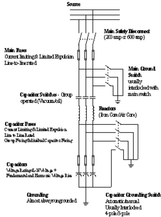
Fig. 1. Typical Medium Voltage Filter Layout
