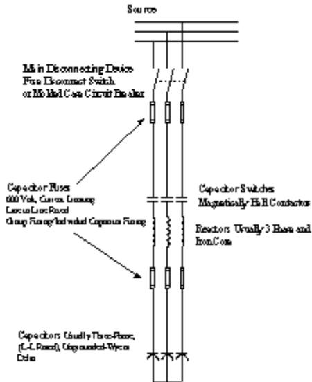
Fig. 2 - Typical Low Voltage Filter Layout
