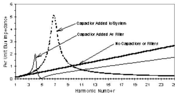
Fig. 6- Harmonic Impedance Scan
